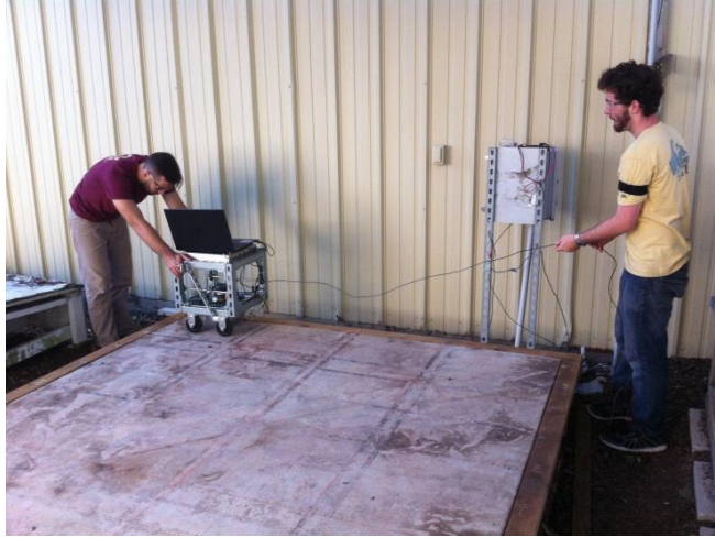
Figure 27-Setup employed when scanning the reinforced concrete slab. The probe operator is seen to the left, and the person holding the trailing wire (right) will eventually be replaced by an automatically spooling wire. At the end of each row the probe was picked up and shifted to the next row and the next scan was initiated.
