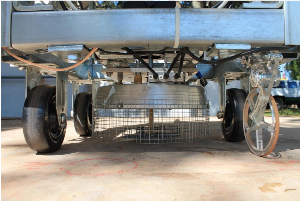
Figure 16- Photo of the underside of the KP. Note the preamplifier (shown with three wires connected), along with the shield and the sensing disk over the concrete.
