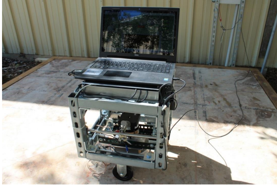
Figure 14- KP on concrete slab with emphasis on Data Processing Unit. Note the following items in the picture, the data processing unit (laptop) and the trailing wire connecting to the rebar mat.
